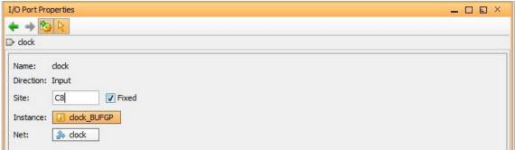
32. The Enable pin needs a switch. I use SW7, which is mapped to pin N3.
