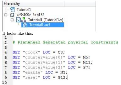
You can see that the .UCF is pretty simple when only working with a few pins. It can be edited directly from here, without using PlanAhead if you want to.
